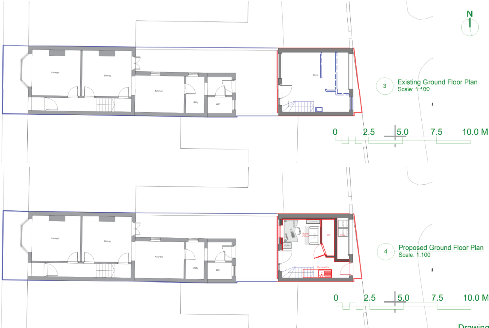
Drawing 002 Existing and Proposed Ground Floor Plans 1:100 @A3 Alterations to Rear of 41 Milton Street, York, YO10 3EP
